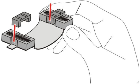
Figure 5-3 AMD CrossFire Installation
